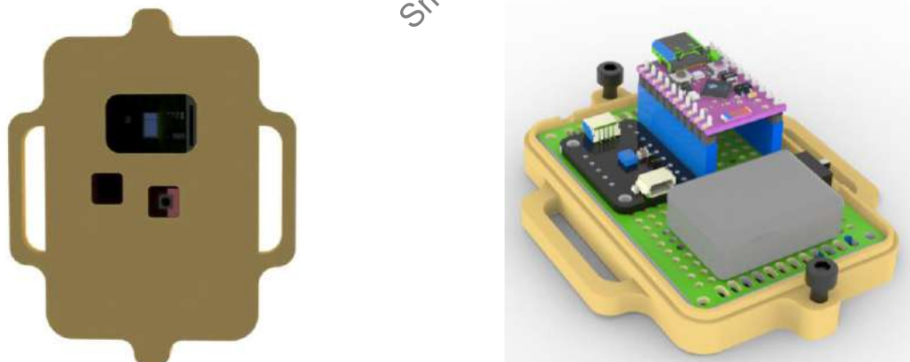
Figure 4 — Main housing: populated board and assembled view
