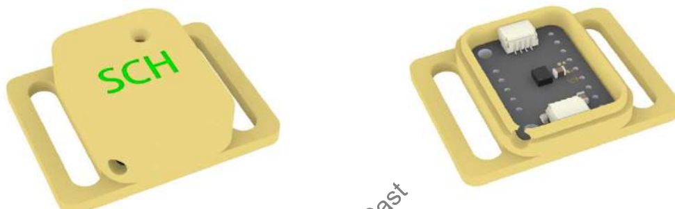
Figure 6 — Second housing containing the upper-arm IMU
